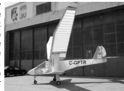
Figure 4. A DeLaurier 2002 flapping wing machine: a synthesis of birds and airplanes. [29]
