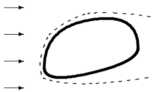
Sketch of the boundary layer around a bluff body in steady uniform flow. On the windward side the boundary layer is thin, whereas it widens and tends to separate on the lee side. In the channel formed by the separated boundary layer, unsteady flow patterns may arise.
