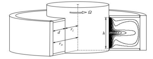
• Flow governed by the incompressible Navier-Stokes equations. In cylindrical coordinates (r, $\theta$ ,z) the non-dimensional Navier-Stokes equations are
