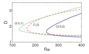
FIG. 3: (Color online) Bifurcation diagram for three pairs of lower/upper-branch equilibrium solutions, with  $(\alpha, \gamma) = (0.5, 1), (0.5, 2)$  and (1, 2). The drag *D* is the wall drag normalized by the drag of laminar flow at the same Reynolds number. For Re = 400, the (0.5, 2)-state has the lowest drag.
