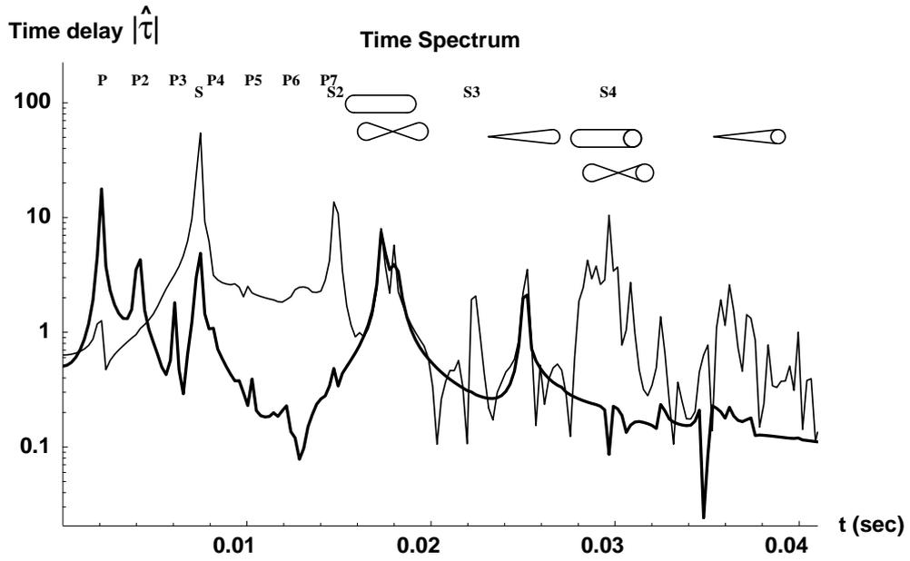
**FIGURE 3.** Power spectrum of cluster fluctuations in time-delay for two cavities. Symbols  $P_i$  and  $S_i$  denote orbits bouncing  $i$  times of pressure respective shear polarization. The circular arcs indicate Rayleigh-surface waves.
