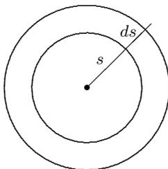
The volume of a spherical shell of thickness  $ds$  and radius  $s$  is  $4\pi s^2 ds$ .
