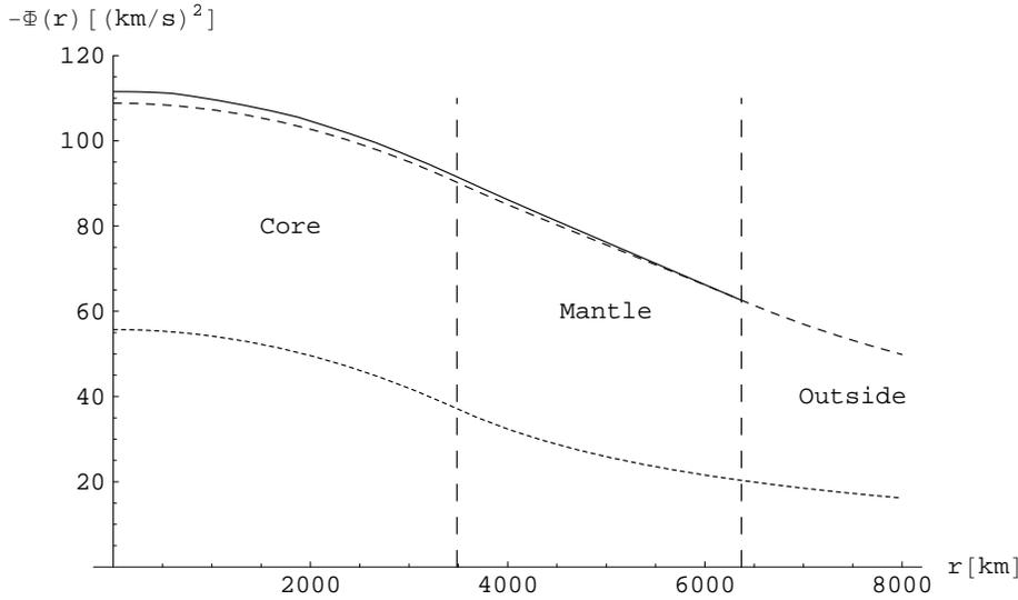
Figure 3.4: The (negative of the) gravitational potential of the Earth as a function of distance from the center. The dotted curve is the potential of the core alone, and the dashed curve is valid for the two-layer model (3-5). The dashed lines indicate the positions of the sharp transitions in the mass density (see fig. 3.1), which have completely disappeared from view in this plot.
