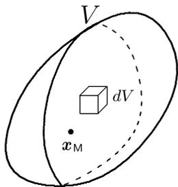
A volume  $V$  with a volume element  $dV$  and center of mass  $\mathbf{x}_M$ .
