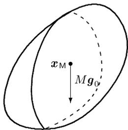
In a constant gravitational field  $\mathbf{g}_0$ , the weight of a body may be viewed as concentrated at the position of the center of mass,  $\mathbf{x}_M$ .
