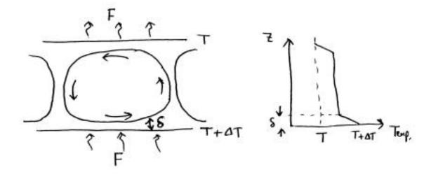
For simplicity, consider free slip top and bottom boundary conditions with heat flow F. At large Prandtl number and high Rayleigh number (but not so high that the convection becomes chaotic), a simple "conveyor belt" picture
