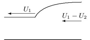
A river bore is obtained by subtracting  $U_1$  from all the velocities of the stationary jump.
