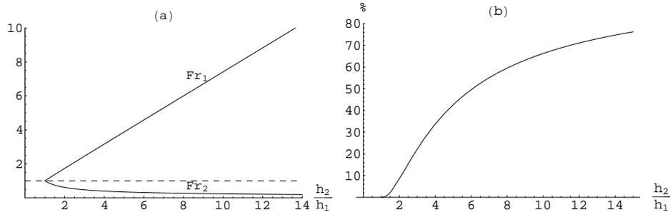
Figure 29.1: **(a)** The Froude numbers  $Fr = U_1/\sqrt{g_0 h_1}$  before and  $Fr_2 = U_2/\sqrt{g_0 h_2}$  after the jump, plotted as function of the height ratio  $h_2/h_1 > 1$ . **(b)** The percentage of the incoming kinetic energy (29-9) dissipated in the stationary jump.
