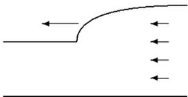
A river bore moving in from the right in water initially at rest. The water behind the front moves slower than the front itself.
