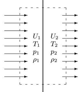
*A piece of a stationary shock front. Fluid comes in from the left with supersonic velocity  $U_1$ , temperature  $T_1$ , pressure  $p_1$  and density  $\rho_1$ . The fluid emerges on the right with subsonic velocity  $U_2$ .*
