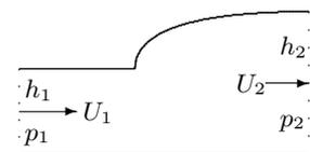
Sketch of an idealized stationary straight-line hydraulic jump of length  $L$  (into the paper). Incompressible fluid enters from the left at velocity  $U_1$  and height  $h_1$  and exits on the right at a lower velocity  $U_2$  and height  $h_2$ . The entry and exit pressures,  $p_1$  and  $p_2$ , are hydrostatic. At the front the flow pattern is complicated, often turbulent. The control volume encompasses the whole drawing between the dotted lines.
