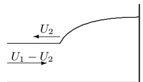
Reflection bore in a closed canal is obtained by subtracting  $U_2$  from all velocities of the stationary jump.
