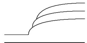
A river bore is “pumped up” by small-amplitude surface waves of sufficiently long wavelenght. Short waves move too slowly to catch up with the jump.
