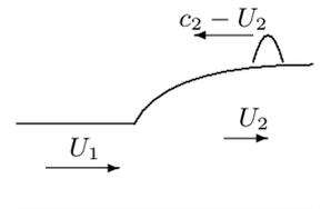
A small amplitude wavelet moving towards the stationary jump with velocity  $c_2 - U_2 > 0$ .
