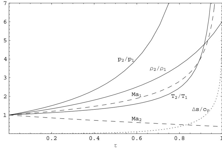
Figure 29.4: The dimensionless Rankine-Hugoniot parameters as function of the relative pressure jump  $\tau$  across the shock. The fully drawn curves are the ratios of pressure, density, and temperature. The dashed curves are the Mach numbers  $Ma_1$  and  $Ma_2$ , and the dotted curve is the specific entropy jump at the shock,  $\Delta s/c_v$  given in (29-22).
