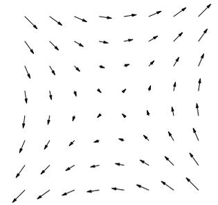
*Plot of the two-dimensional linear displacement field  $\mathbf{u} = (\alpha y, \alpha x, 0)$  for  $-1 < x < 1$  and  $-1 < y < 1$ . The material is dilated along one diagonal and contracted along the other. These are the principal directions of strain (see problem 9.8).*
