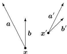
Displacement of a pair of infinitesimal material needles may affect their lengths as well as the angle between them.
