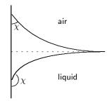
An air/liquid interface meeting a wall. The upper curve makes an acute contact angle, like water, whereas the lower curve makes an obtuse contact angle, like mercury.
