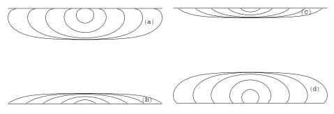
Figure 8.2: Shapes of stable air bubbles and droplets of water ( $R_c = 2.7 \text{ mm}, \chi_c = 1^\circ$ ) and mercury ( $R_c = 1.9 \text{ mm}, \chi_c = 140^\circ$ ). (a) Air bubbles in water under a lid (to scale). (b) Water droplet on table plotted with vertical scale enlarged 40 times. (c) Air bubbles in mercury (to scale). (d) Mercury droplets on a table (to scale).
