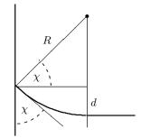
Approximatively circular geometry of a liquid surface with acute contact angle near a vertical wall.
