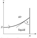
For the capillary with acute angle of contact both centers of curvature lie outside the liquid.
