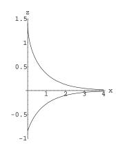
Capillary surface shape of water and mercury in units where  $R_c = 1$ . Notice the exaggerated vertical scale.
