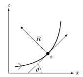
The geometry of a planar curve. The curve is parameterized by the arc length s along the curve. A small change in s generates a change in the elevation angle  $\theta$  determined by the local radius of curvature. Here the radius of curvature is positive.
