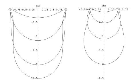
Figure 8.3: Static droplet shapes at the mouth of a circular tube in units of  $R_c = 1$ . There are no solutions with larger volumes than the largest ones shown here. All contact angles are assumed to be possible at the mouth of the tube. (a) Tube with radius a = 1which is larger the critical radius ( $a_1 = 0.918$ ). (b) Tube with radius a = 0.5 which is smaller than the critical radius.
