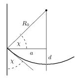
Approximatively spherical surface with acute contact angle in a circular tube.
