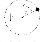
Inverted mathematical pendulum with angle  $\theta$  moving towards the unstable equilibrium at  $\theta = 0$ . This sketch corresponds to a liquid with acute contact angle. If the contact angle is obtuse, the pendulum has to start from the other side of the unstable equilibrium.
