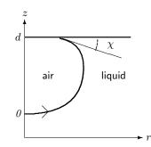
An air bubble in under a horizontal lid with acute angle of contact.
