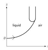
A liquid drop hanging from a tube. Any contact angle can be accommodated by the  $180^{\circ}$  turn at the end of the tube's material.
