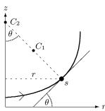
The interface curve is parameterized by the arc length s. A small change in s generates a change in the elevation angle  $\theta$  determined by the local radius of curvature  $R_1$  with center  $C_1$ . The second radius of curvature  $R_2$  lies on the z-axis with center  $C_2$  (see problem 8.3).
