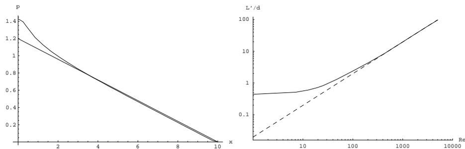
Figure 21.6: The pressure is shown on the left as a function of distance  $x$  from the entrance. Its gradient becomes constant at about  $x = 2.5$ . The (95%) entrance length is plotted as a function of Reynolds number on the right. The dashed line corresponds to  $L'/d = k Re$  with  $k = 0.0197$ . For  $Re \lesssim 10$  the curve approaches the constant value 0.43.
