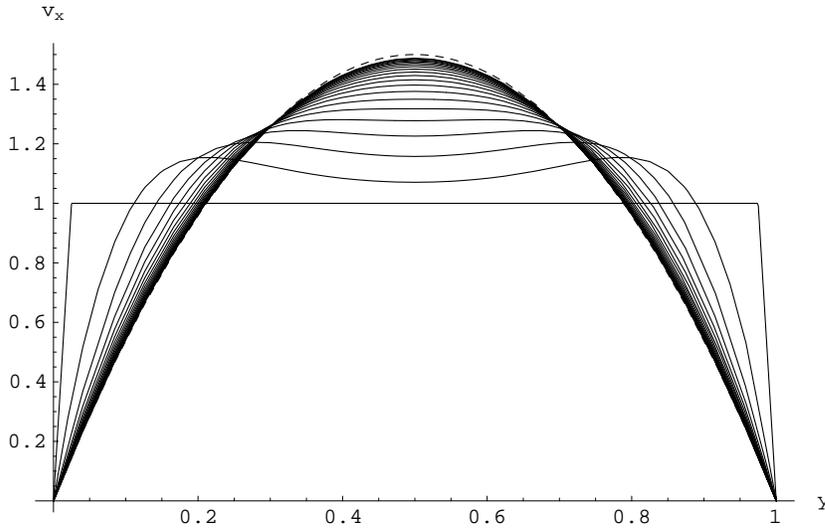
Figure 21.4: Transformation of the steady velocity profile from the initial square shape to the parabolic Poiseuille shape (dashed) downstream from the entrance. The Reynolds number is chosen to be  $\text{Re} = 100$ , the channel length  $L = 10$  and width  $d = 1$ , and the curves are separated by  $\Delta x = 1/N_x$  (with  $N_x = 40$ ) in the interval  $0 \leq x \leq L/2$ .
