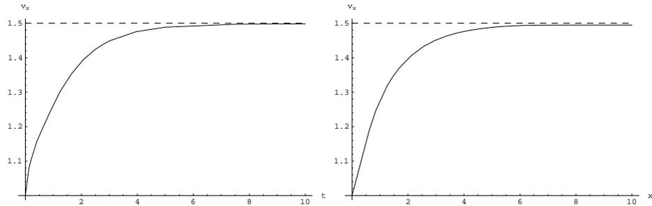
Figure 21.5: The graph on the left shows the rise of the exit velocity  $v_x(L, d/2, t)$  as a function of time, whereas the graph on the right shows the steady state velocity along the middle of the channel  $v_x(x, d/2)$  as a function of  $x$ . The Reynolds number is 100. Both curves approach the Poiseuille maximal velocity of 1.5 times the average velocity.
