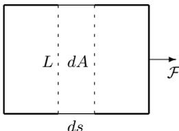
An external force  $\mathcal{F}$  performs the work  $dW = \mathcal{F} ds$  to stretch the surface by  $ds$ . Since the area increase is  $dA = Lds$ , the force is  $\mathcal{F} = \alpha L$ . The force per unit of length,  $\alpha = \mathcal{F}/L$ , is the surface tension.
