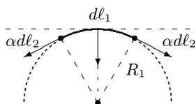
The rectangular piece of the surface of size  $dl_1 \times dl_2$  is exposed to two tension forces along the 1-direction resulting in a normal force pointing towards the center of the circle of curvature. The tension forces in the 2-direction also contribute to the normal force.
