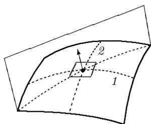
A plane containing the normal in a point intersects the surface in a planar curve with a signed radius of curvature in the point. The extreme values of the signed radii of curvature define the principal directions. The small rectangle has sides parallel with the principal directions.
