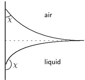
*An air/liquid interface meeting a wall. The upper curve makes an acute contact angle, like water, whereas the lower curve makes an obtuse contact angle, like mercury.*
