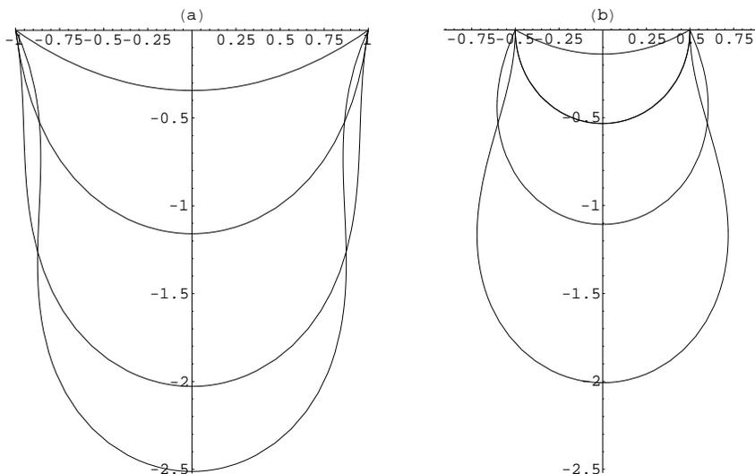
Figure 8.3: *Static droplet shapes at the mouth of a circular tube in units of  $R_c = 1$ . There are no solutions with larger volumes than the largest ones shown here. All contact angles are assumed to be possible at the mouth of the tube. (a) Tube with radius  $a = 1$  which is larger the critical radius ( $a_1 = 0.918$ ). (b) Tube with radius  $a = 0.5$  which is smaller than the critical radius.*
