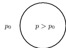
*Surface tension increases the pressure inside a spherical droplet or bubble.*
