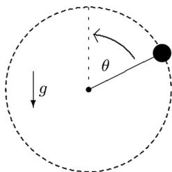
*Inverted mathematical pendulum with angle  $\theta$  moving towards the unstable equilibrium at  $\theta = 0$ . This sketch corresponds to a liquid with acute contact angle. If the contact angle is obtuse, the pendulum has to start from the other side of the unstable equilibrium.*
