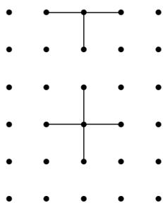
Two-dimensional cross section of a primitive three-dimensional model of a material interfacing to vacuum. A molecule at the surface has only five bonds compared to the six that tie a molecule in the interior.
