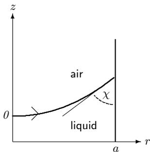
For the capillary with acute angle of contact both centers of curvature lie outside the liquid.
