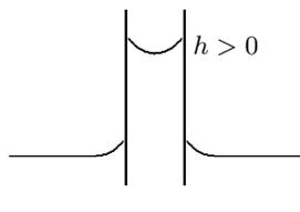
Water rises above the ambient level in a glass tube and displays a concave surface inside the tube. Mercury behaves oppositely and sinks with a convex surface.
