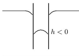
Mercury sinks below the general level in a capillary glass tube.
