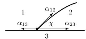
*Two fluids meeting at a solid wall in a line orthogonal to the paper. The tangential component of surface tension must vanish.*
