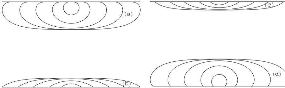
Figure 8.2: Shapes of stable air bubbles and droplets of water ( $R_c = 2.7$  mm,  $\chi_c = 1^\circ$ ) and mercury ( $R_c = 1.9$  mm,  $\chi_c = 140^\circ$ ). (a) Air bubbles in water under a lid (to scale). (b) Water droplet on table plotted with vertical scale enlarged 40 times. (c) Air bubbles in mercury (to scale). (d) Mercury droplets on a table (to scale).
