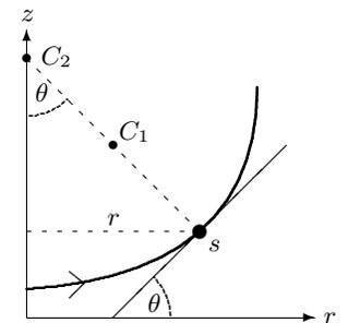
The interface curve is parameterized by the arc length  $s$ . A small change in  $s$  generates a change in the elevation angle  $\theta$  determined by the local radius of curvature  $R_1$  with center  $C_1$ . The second radius of curvature  $R_2$  lies on the  $z$ -axis with center  $C_2$  (see problem 8.3).
