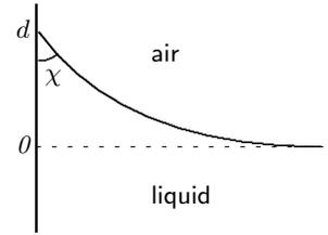
The interface at a vertical wall with an acute angle of contact.
