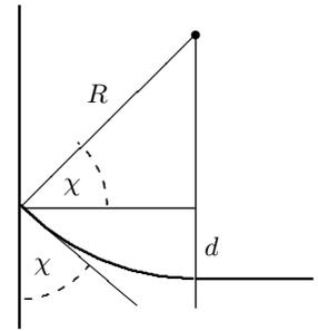
Approximately circular geometry of a liquid surface with acute contact angle near a vertical wall.
