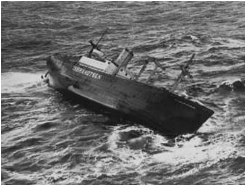
Figure 3.2. The Flying Enterprise (1952). A body can float stably in many orientations, depending on the position of its center of gravity. In this case the list to port was caused by a shift in the cargo which moved the center of gravity to the port side. The ship and its lonely captain Carlsen became famous because he stayed on board during the storm that eventually sent it to the bottom. Photograph courtesy Politiken , Denmark, reproduced with permission.
