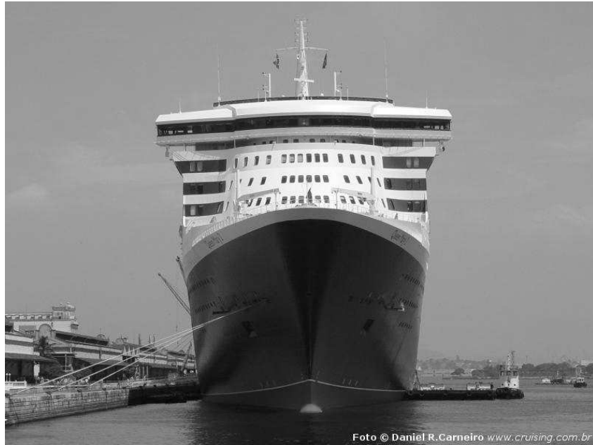
Figure 3.3. The Queen Mary 2 set sail on its maiden voyage on January 2, 2004. It was at that time the world's largest ocean liner with a length of 345 m, a height of 72 m from keel to funnel, and a width of 41 m. Having a draft of only 10 m, its superstructure rises an impressive 62 m over the waterline. The low average density of the superstructure, including 2620 passengers and 1253 crew, combined with the high average density of the 117 megawatt engines and other heavy facilities close to the bottom of the ship nevertheless allow the stability condition (3.28) to be fulfilled. Photograph by Daniel Carneiro.
