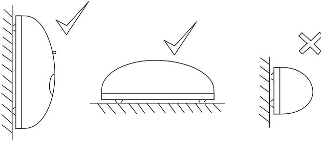
If you have a float-free Precision 406 it is critical that you choose a position where the released EPIRB will **not get trapped by overhangs, rigging, antennas** etc, should the vessel ever sink. An expanse of flat surface is required to allow the enclosure lid to eject. Use the list below to choose a suitable mounting position:
