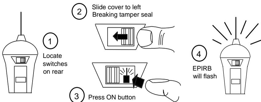
Once activated the Precision 406 **must** have its antenna near upright and it must have a clear view of the sky for proper operation. Lying it on its side or placing it next to a metal wall will impair its range and may fail to alert the rescue services. Avoid handling the antenna, as this will also impair performance.
