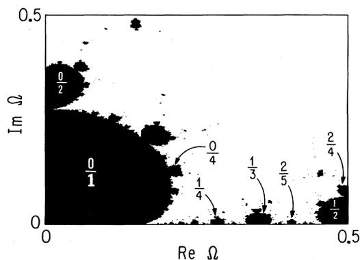
FIG. 3. Mode locking in the complexified circle map. Plotted is the complex  $\Omega$  plane and in the black regions the iterations are mode locked. The real axis has the same structure as Fig. 1.
