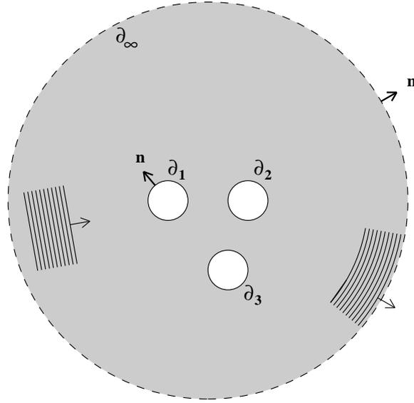
**FIGURE 1.** General zone of two-dimensional cavity scattering.
