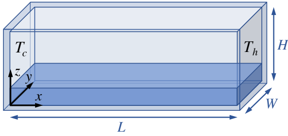
FIG. 1. The test cell containing the liquid and air/vapor mixture. Gravity is pointing in the negative z direction. The shape of the contact line reflects the curvature of the free surface for a liquid wetting the walls. The inner dimensions are H = W = 10 mm, L = 48.5 mm, the walls are 1.25 mm thick, and the liquid (gas) layer has a thickness d_l = 2.5 mm ( d_g = 7.5 mm).
