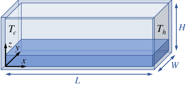
Figure 1: A sealed test cell containing the liquid and air/vapor mixture. Gravity is pointing in the negative z direction.
