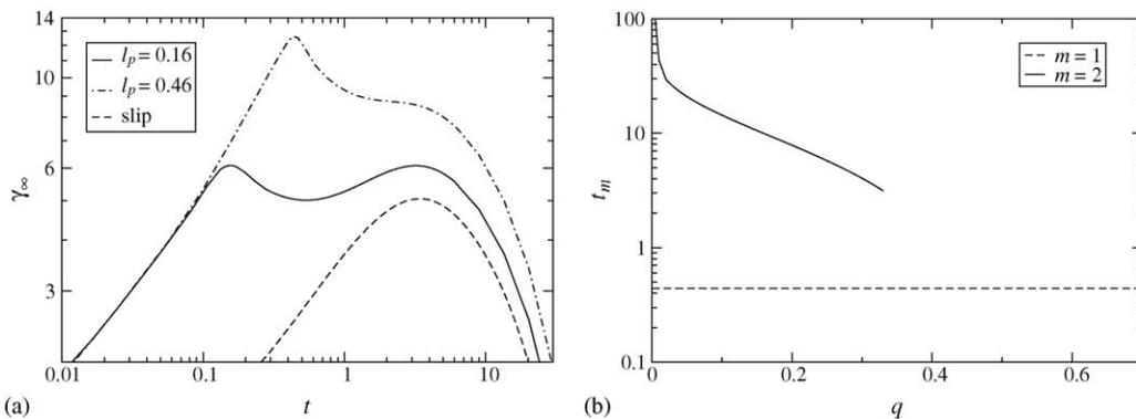
Fig. 5. (a) Transient amplification  $\gamma_\infty$  at  $q = 0.36$  for the slip and precursor model as a function of time. The width of the numerical precursor film is as indicated. (b) The times at which the maxima in  $\gamma_\infty$  are achieved as a function of wave number in the precursor model with  $l_p = 0.46$ . The second maximum disappears at larger wave numbers. The other parameters are  $D = 5$ ,  $\alpha = b = 0.01$  and  $c = 1.303$ .
