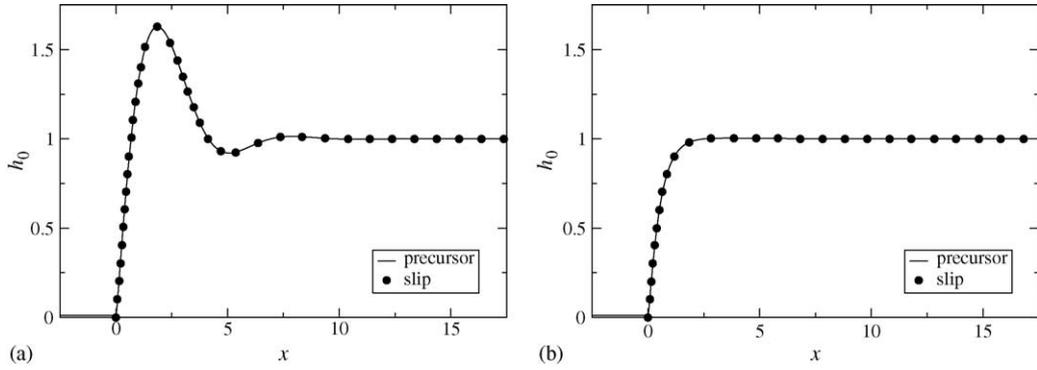
Fig. 1. Asymptotic film thickness profiles produced by the two models for  $b = \alpha = 0.01$  and (a)  $D = 0$  ( $90^\circ$  inclination angle) or (b)  $D = 5$  ( $10^\circ$  inclination angle). The contact angle in the slip model is chosen to obtain the maximal thickness equal to that produced by the precursor model: (a)  $c = 1.236$  and (b)  $c = 1.303$ .
