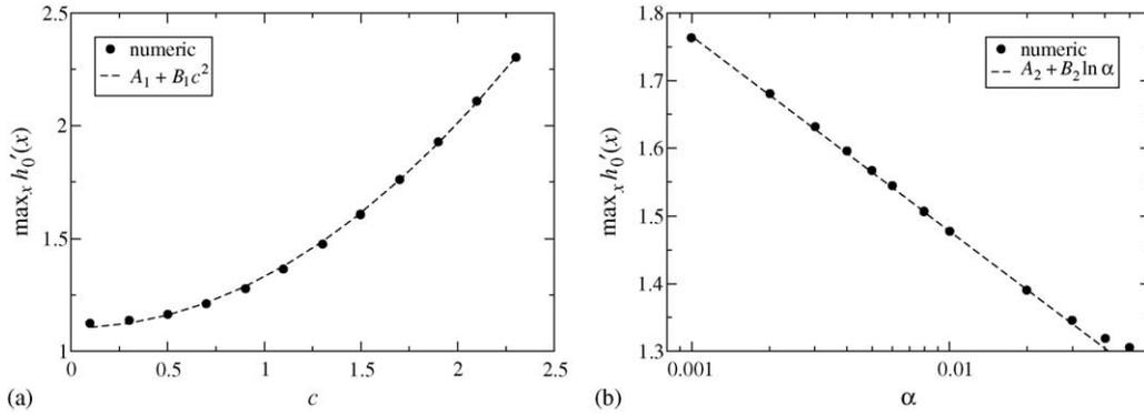
Fig. 9. The maximal slope of the capillary shock (a) as a function of the contact angle for  $\alpha = 0.01$  and  $D = 5$  and (b) as a function of the slip parameter for  $c = 1.303$  and  $D = 5$ .  $A_i$  and  $B_i$  are constants determined from a least squares fit.
