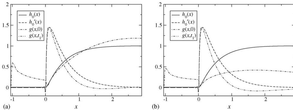
Fig. 8. Optimal initial disturbance  $g(x, 0)$  that produces the largest disturbance  $g(x, t)$  at the peak time  $t_1$  for (a)  $q = 0$  and (b)  $q = 0.6$ . The other parameters are  $D = 5$ ,  $b = 0.01$  and  $l_p = 1.06$ .
