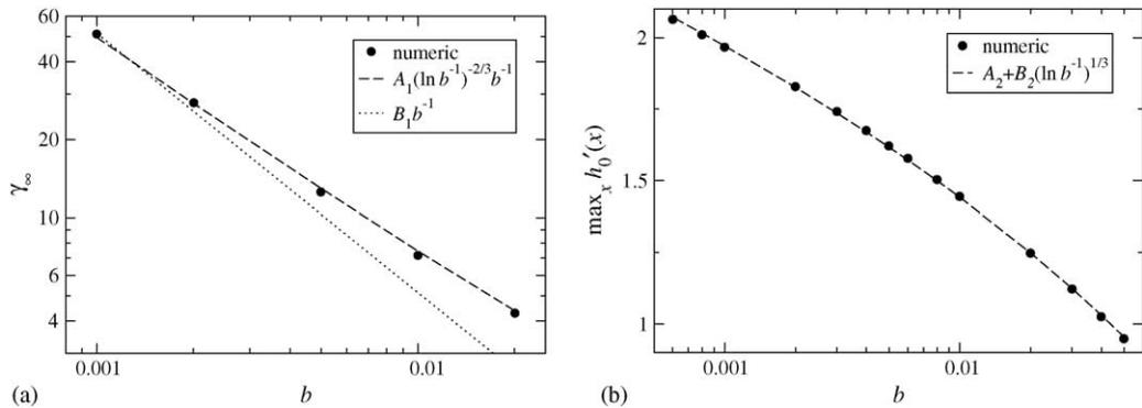
Fig. 7. (a) Transient amplification  $\gamma_\infty$  for  $q = 0.6$  and (b) the maximal slope of the capillary shock as a function of the precursor thickness  $b$ . The other parameters are  $D = 5$ ,  $b = 0.01$  and  $l_p = 0.2$ .  $A_i$  and  $B_i$  are constants determined from a least squares fit.
