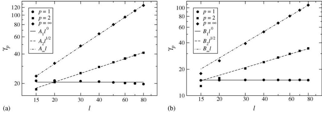
Fig. 4. Maximal transient amplification  $\gamma_p$  at  $q = 0$  as a function of the system size  $l$  for (a)  $D = 0$  and (b)  $D = 5$ . The other parameters are as in Fig. 1.  $A_i$  and  $B_i$  are constants determined from a least squares fit.
